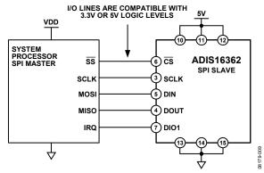
Figure 9. Electrical Connection Diagram
