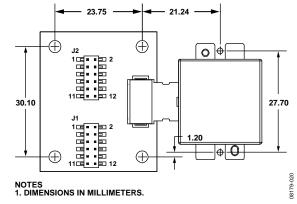
Figure 16. Physical Diagram for the ADIS16362/PCBZ
