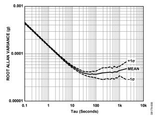
Figure 8. Accelerometer Allan Variance
