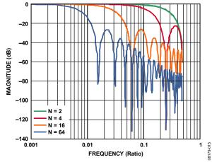
Figure 14. Bartlett Window, FIR Filter Frequency Response (Phase Delay = N Samples)
